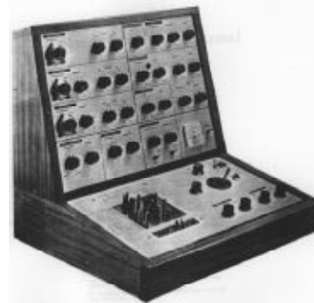
Fig. 7. A 1970 VCS-3 Putney. Although a small keyboard could be attached to it, it was often played by turning knobs.
